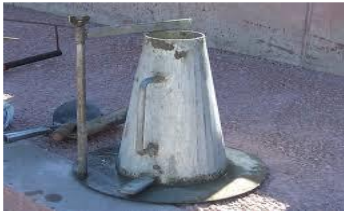
Fig. slump flow test in progress
