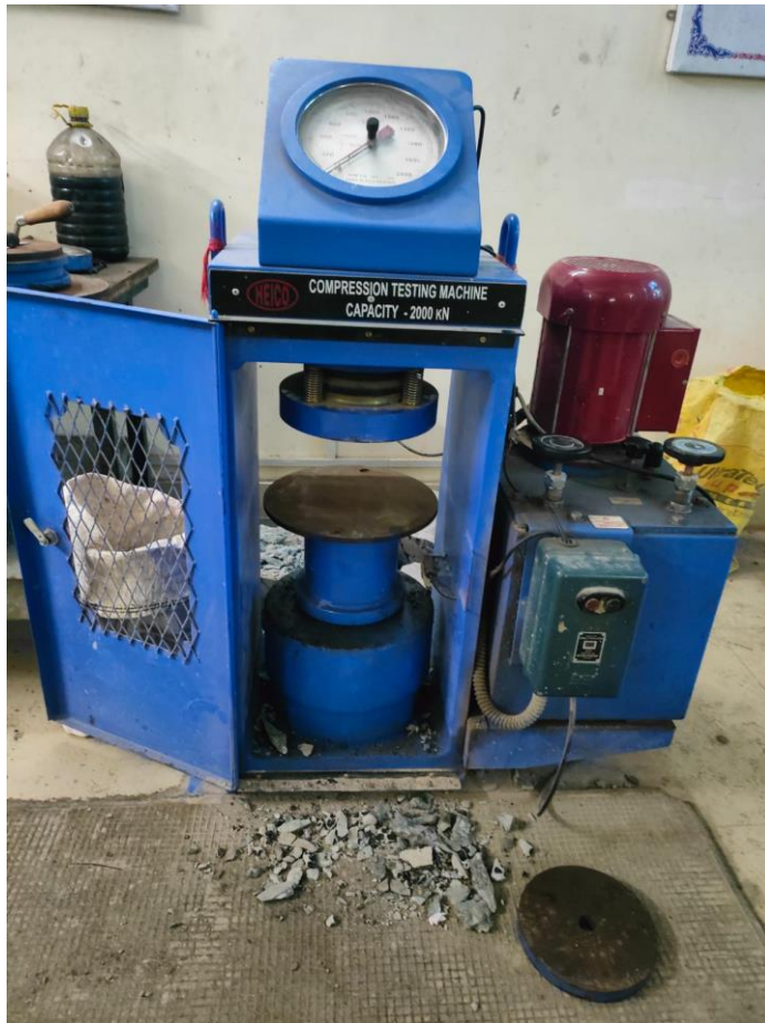
Figure 4.8- Compressive Strength Test Of Cube in CTM
