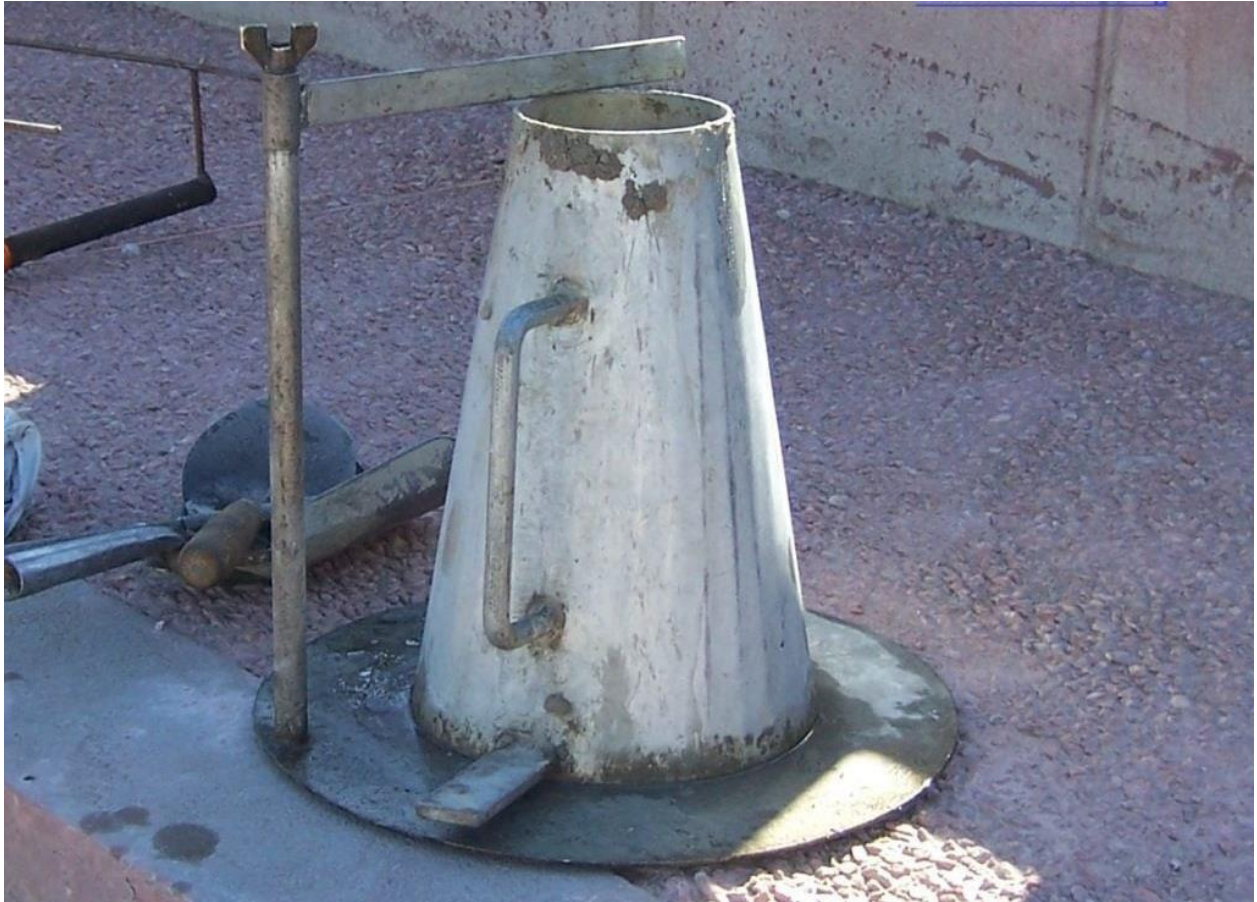
Fig 4.1 Slump Flow Test In Progress
