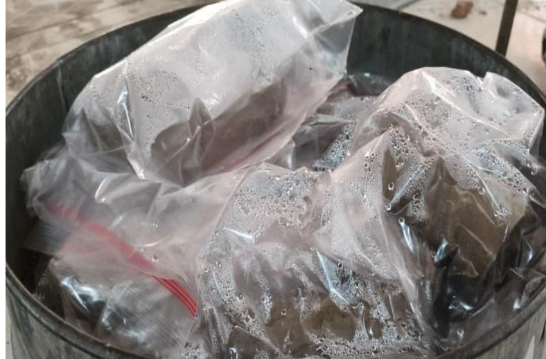
Fig 3.3 Curing of soil sample for UCS test
