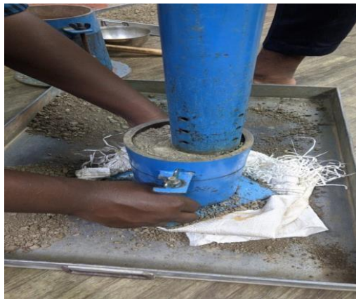
Fig 3.6 Modified proctor test (Heavy compaction)
