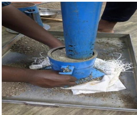
Fig 3.5 Modified proctor test (Heavy compaction)
